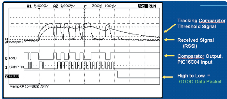
Figure 2. A good RSSI signal and the corresponding comparator output that reconstructs the received serial data stream.
